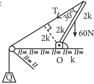
$$\begin{aligned} \vec{\Sigma M}_O &= \vec{0} \\ -60 \cdot k + T \cdot 2k &= 0 \\ T &= 30 \text{ N} \\ \Rightarrow F_Q &= 30 \text{ N} \\ m_Q g &= 30 \\ m &= 3 \text{ kg} \end{aligned}$$
