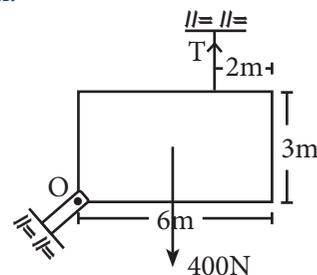
$$\begin{aligned} \sum \vec{M}_O^F &= \vec{0} \\ T \cdot 4 - 400 \cdot 3 &= 0 \\ T &= 300 \text{ N} \end{aligned}$$
