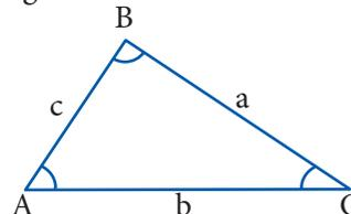
$$a = b \text{ Cos}C + c \text{ Cos}B \quad b = a \text{ Cos}C + c \text{ Cos}A$$
